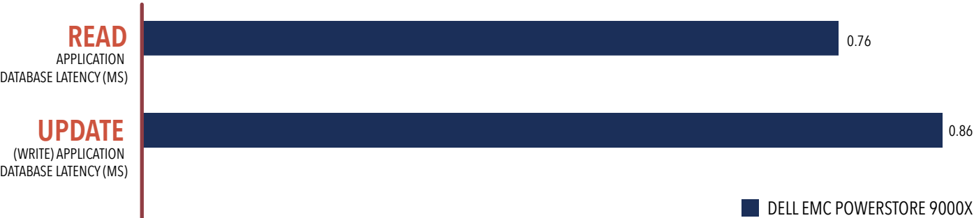
Figure 5: Application latency (ms) delivered by the Dell EMC PowerStore 9000X while hosting internal VMs and simultaneously delivering storage to internal hosts. Vendor A cannot host internal VMs, so we could not make a comparison. Lower is better. Source: Principled Technologies.
